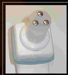
Fig. 4 Head of the electric device used to perform pulsed current iontophoresis. Actual size: 30 mm dia
